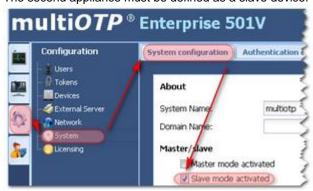
The slave appliance will **not** synchronize with the defined AD/LDAP server, except if the master is down for at least twice the AD/LDAP synchronization time, the slave will synchronize with the AD/LDAP server. The slave appliance will **not** send automatic provisioning emails.
